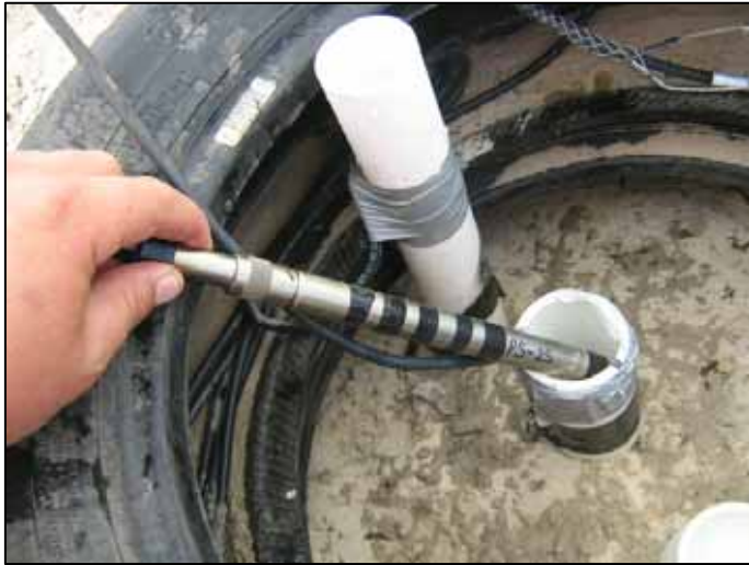
Plates 14-15. Installation of groundwater (piezometric) levels sensors.
