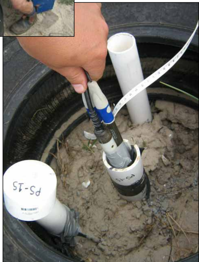
Plates 22-23. Field measurement of general water quality parameters at multiple depths in the sediment profile.
