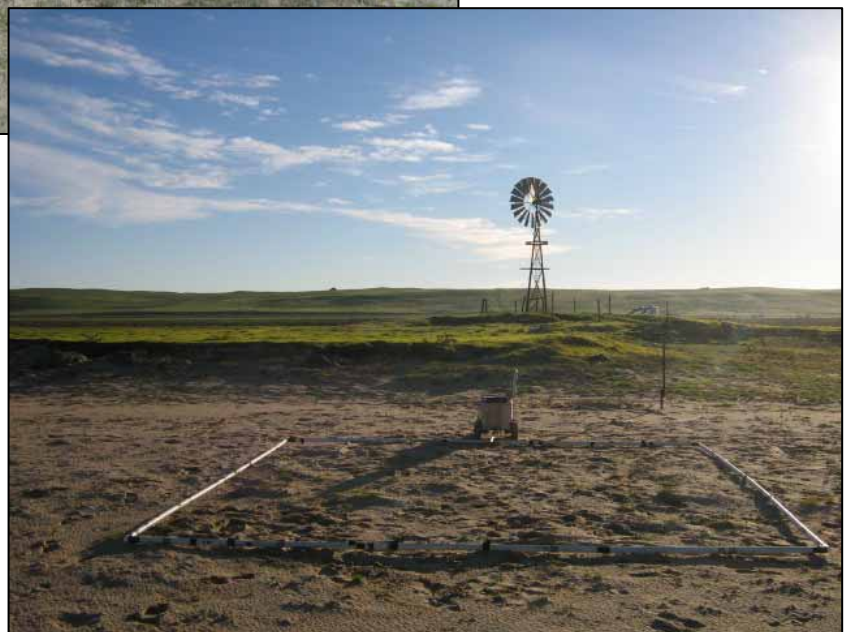
Plates 5-6. Geophysical surveys were conducted across the exposed shoreline sediments of Lake Alexandrina (Point Sturt) and Lake Albert (Campbell Park, Meningie and Windmill locations). Survey apparatus at Point Sturt and Windmill locations pictured above.
