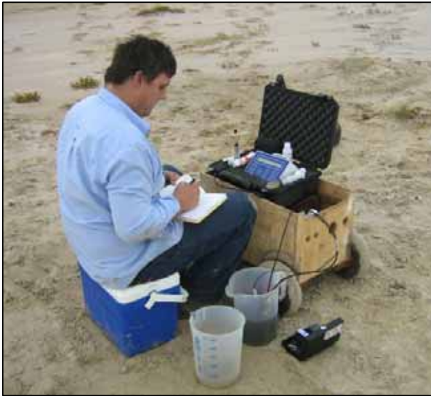
Plates 26-28. Field measurement of general water quality parameters (left) and acidity/alkalinity (below).
