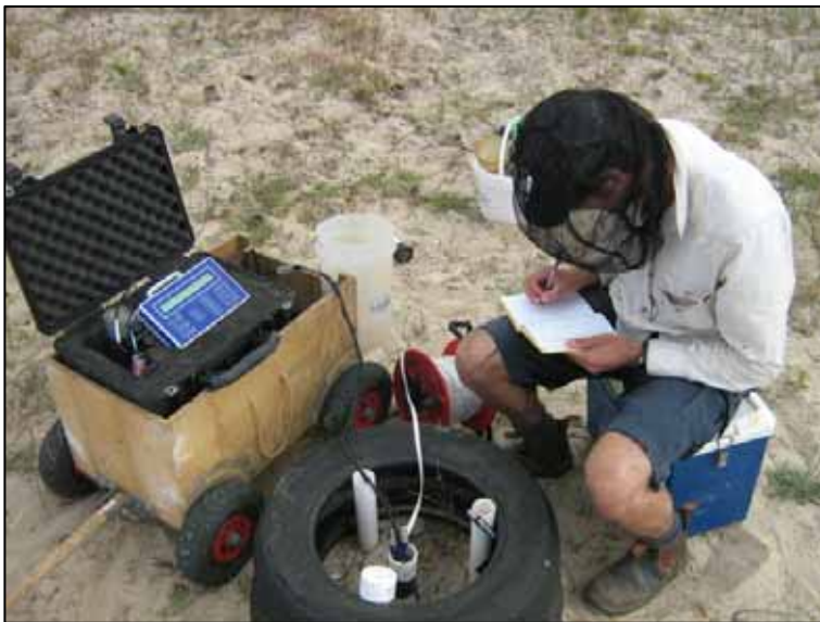
Plates 22-23. Field measurement of general water quality parameters at multiple depths in the sediment profile.
