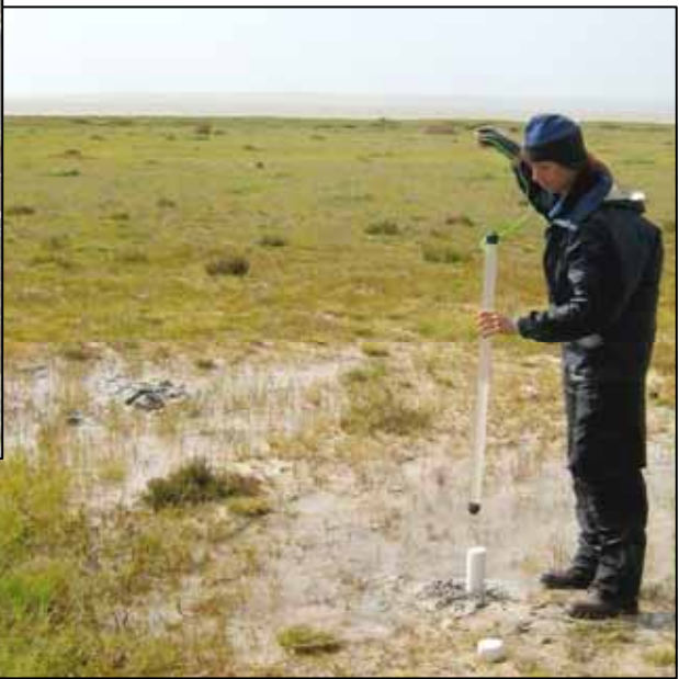
Plates 24-25. Collection of bulk groundwater samples for laboratory analysis.
