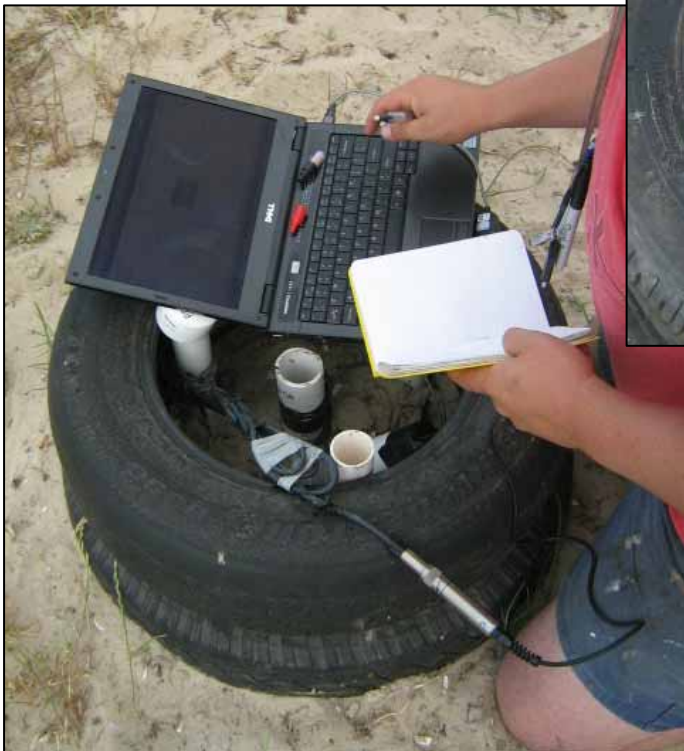
Plate 16. Data download from groundwater (piezometric) levels sensors.
