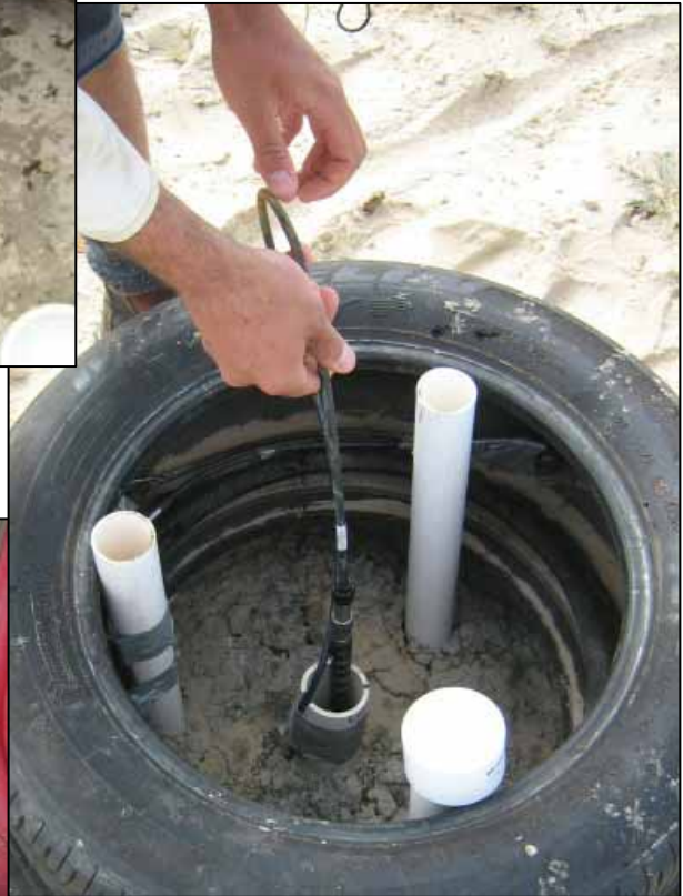
Plates 14-15. Installation of groundwater (piezometric) levels sensors.
