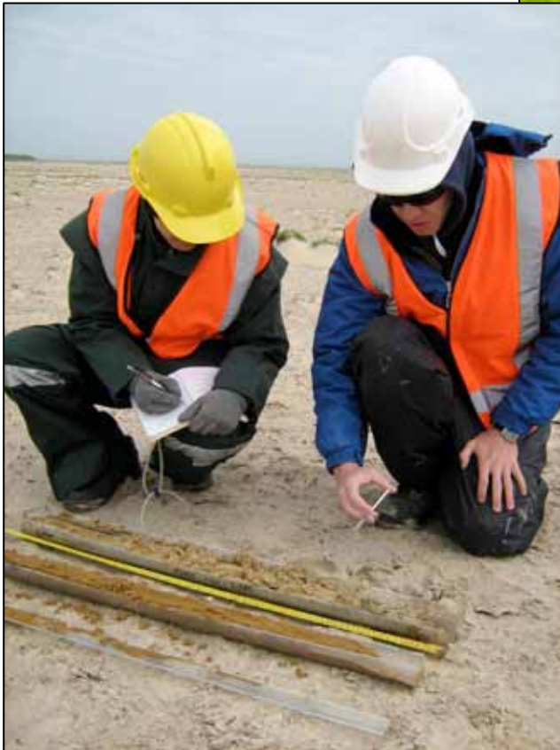
Plate 4. Logging of push-tube samples to determine the local geology and assist with ground-truthing of geophysical survey data, piezometer site confirmation and detailed piezometer design (e.g. screened zone location and extent).
