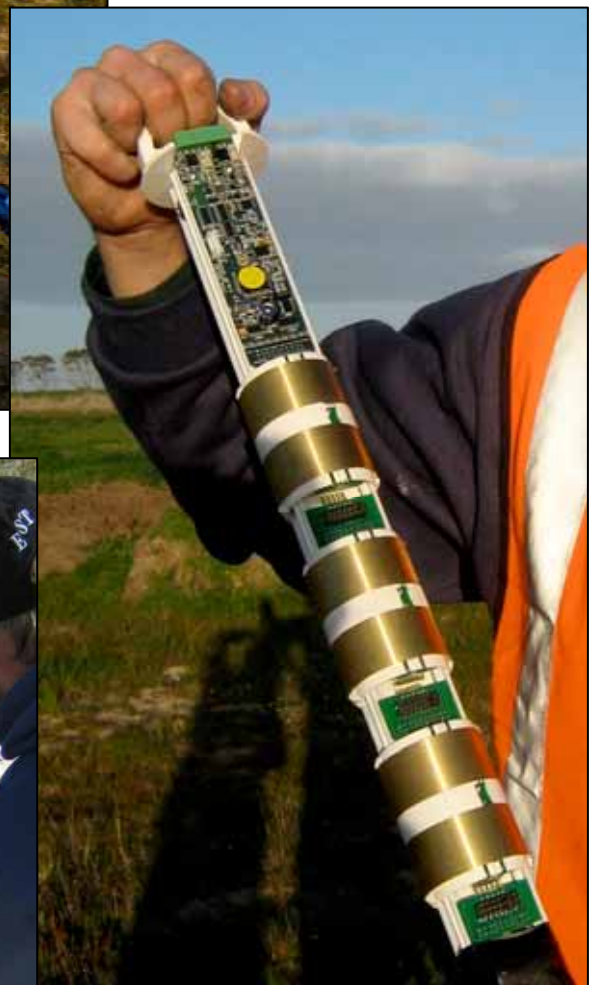
Plate 20. Moisture probe comprising data logging facility and 3 moisture sensors spaced at 10 cm vertical intervals in preparation for installation at Campbell Park (August 2009). Two additional sensors were installed in September 2009.
